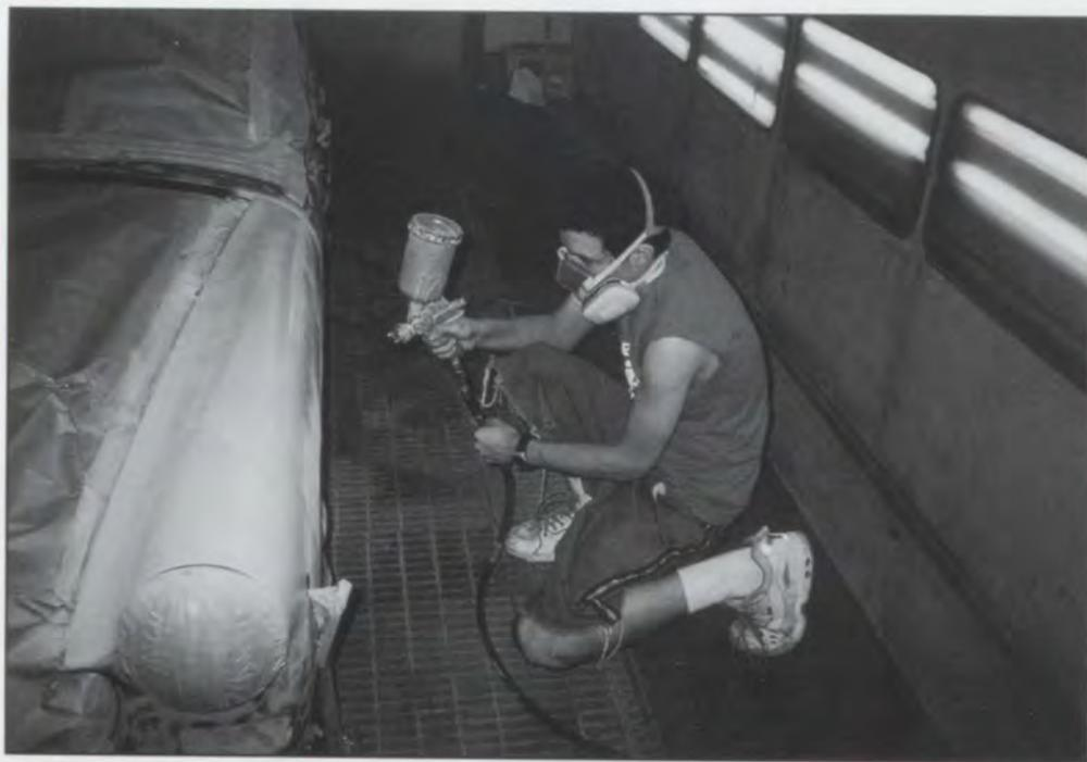
Using the paint booth in Dauby's Body Shop, Seth Adams works with Jared Feltner while priming an MG convertible. They put on three coats of primer before applying the top coat.
